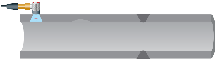
Conventional UT provides localized inspection, underneath or in the vicinity of the probe location.
